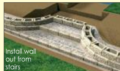
Install next stair riser
