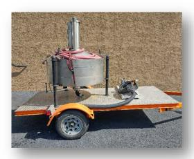
Trailer Mounted 100 Gallon LPG Prover LPG Meter Calibration 20 - 100 GPM Flow Rates
